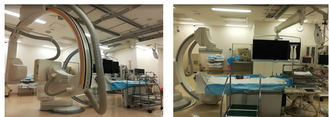
Figure 1. Biplane angiography system (Artis Zee, Siemens, Germany) in Hyogo College of Medicine, Japan.
